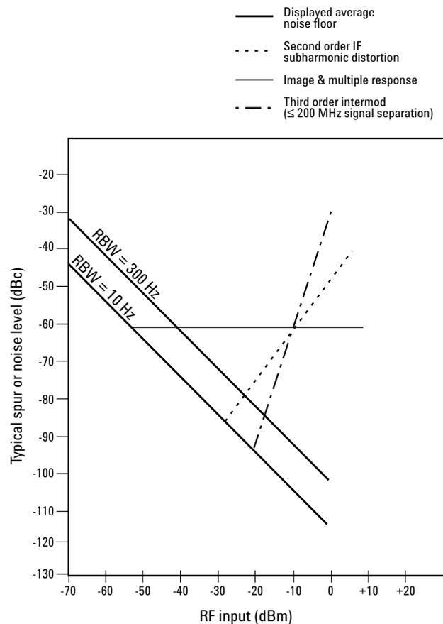
Figure 3. Agilent 11974A System Dynamic Range
