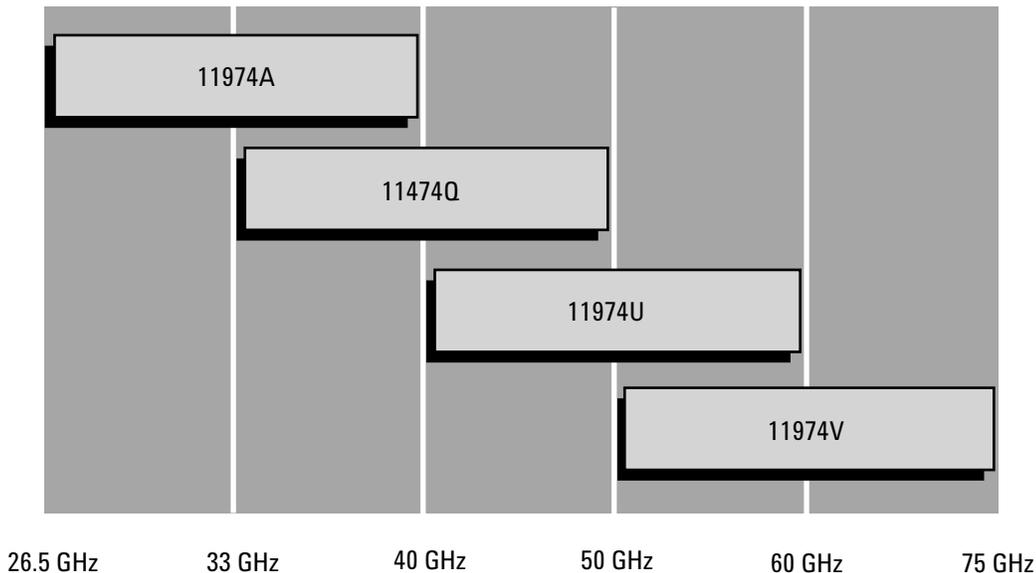
1. Operation with 8566B spectrum analyzers requires the use of an 11975A LO amplifier to provide sufficient local oscillator power to the 11974 series LO input.
