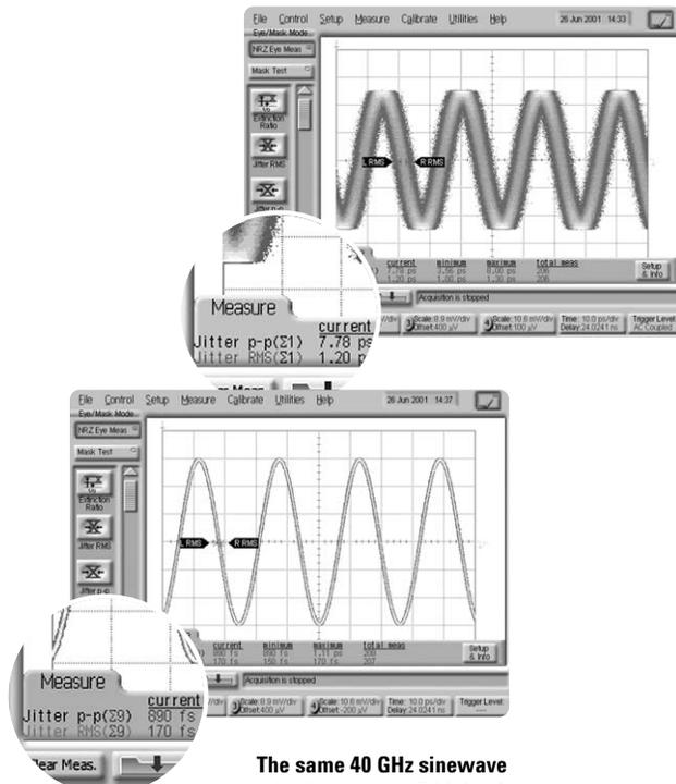
The same 40 GHz sine wave captured using current DCA (top) and now with 86107A precision timebase module (bottom).
