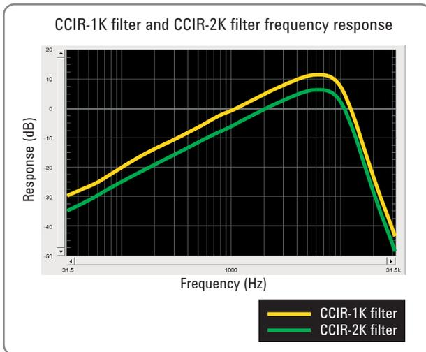
Figure 16. CCIR-1K filter and CCIR-2K filter frequency response
