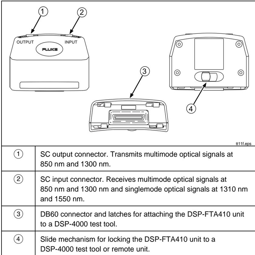
**Figure 2. Features of the DSP-FTA410 Fiber Test Adapter**
