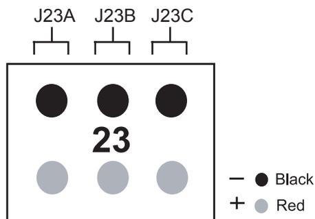
Figure 1: Labels for a jar with 6 posts
