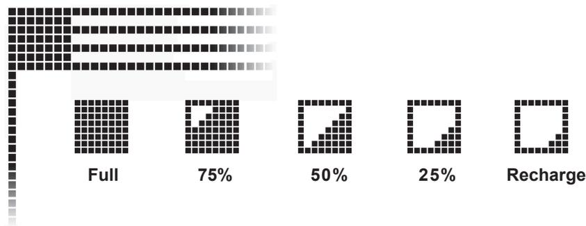
Recharge the analyzer battery pack if:
