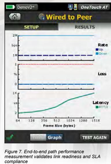
Figure 7. End-to-end path performance measurement validates link readiness and SLA compliance
