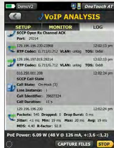
Figure 9. Inline VoIP analysis simplifies troubleshooting of desktop VoIP problems in real-time without TAPs or switch mirror ports
